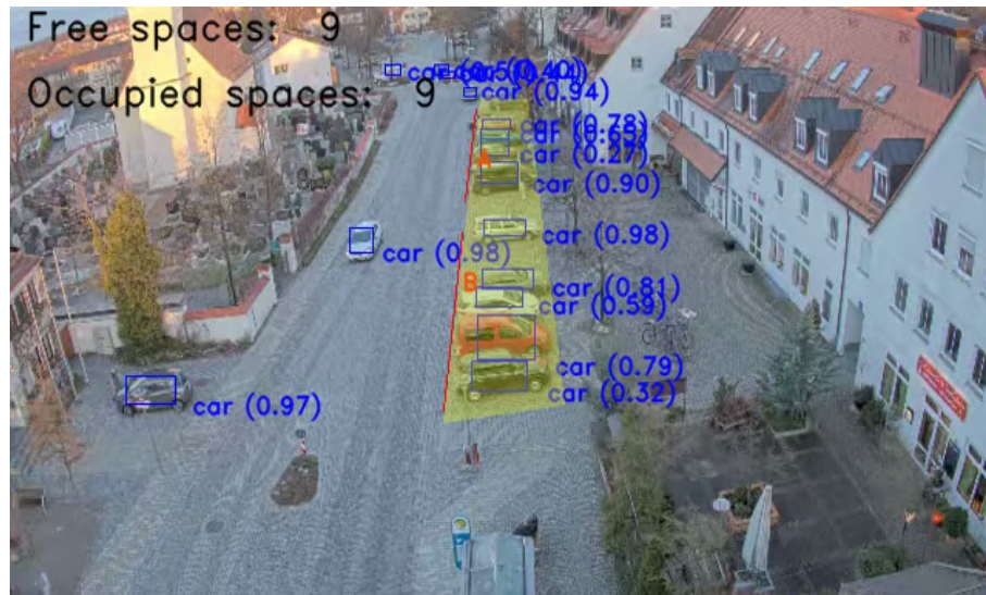
Figure 11: Before retraining: 9/11 cars detected on the parking area
